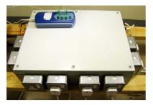
The products under test are connected to the UMS Test system which has full data control and recording using Labview software. This allows full integration of the Test equipment used - Kikusui AC Stable Power Supply , Yokogawa Power Analyser, Pico Temperatrure Logger and a LUX-TSI distribution control panel
