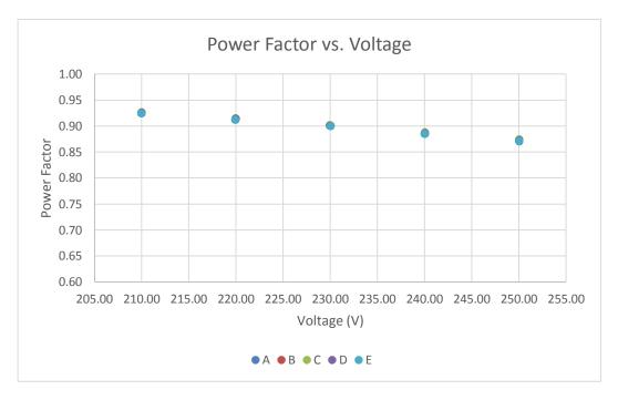
Power factors measured have a Leading phase angle and therefore the driver has capacitive properties.
