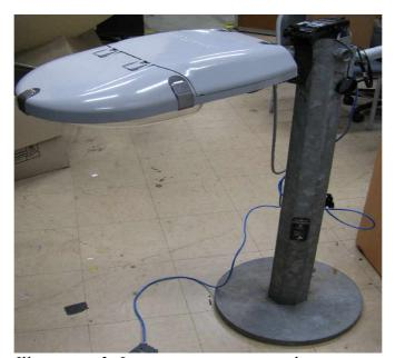
Illustration 3: Luminaire setup on a pole
